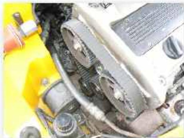
Whilst the front suspension was out I took the opportunity to replace the cam belt. Not a job I what to do again in a hurry. I fitted new belts to power steering and alternator. The turbo and exhaust heat shields were removed and re-plated and most of the visible bolts were replaced with stainless steel. That was the engine bay done.
