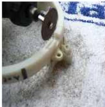
Bits had a tested used unit in the post. Another issue was 2 rusty lamps. These were quite easy to find although I had to modify the white plastic ring to fit the ones I found. I used a Dremel to cut a slot in the plastic ring to take the lugs on the back of the lamps. The module arrived the next day and was promptly fitted, still I had no lights. Back to Elan Central and a long look at the
