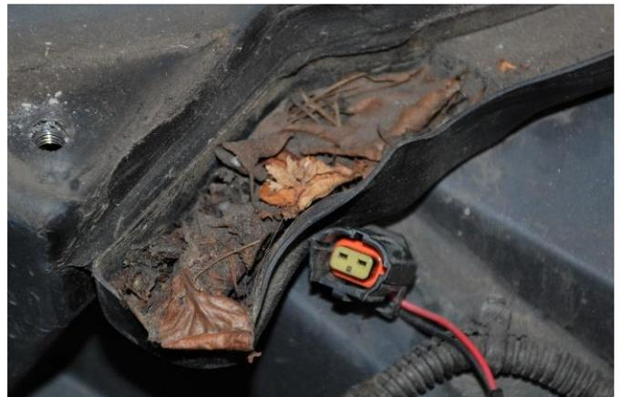
(3) – Blocked hidden scuttle drain channel
