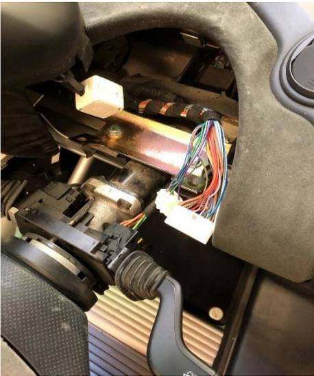
Instruments & module removed
