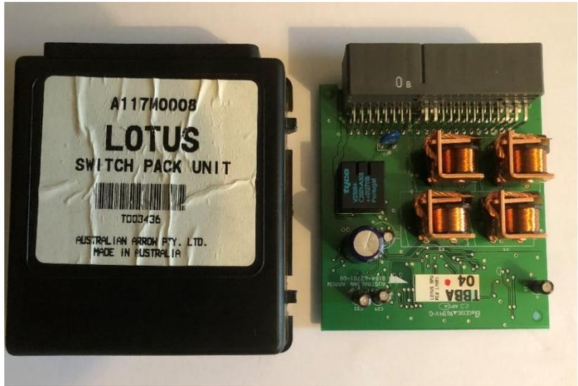
Plug in Elise Lighting Control Module Box & Circuit board
