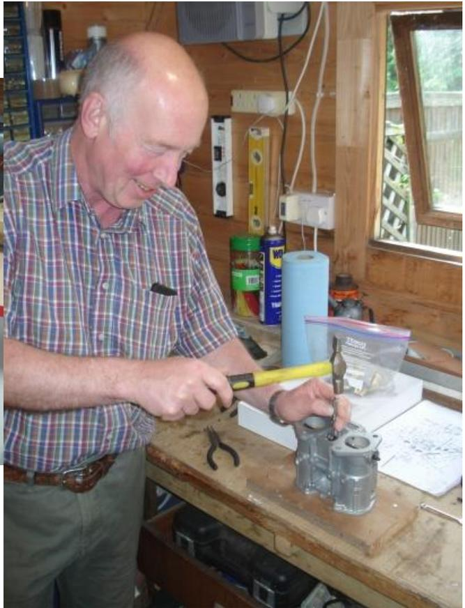
Note how well the components came up after vapour blasting. I sourced replacement parts from Eurocarbs which has an excellently detailed website in terms of drawings, photos and parts identification.
