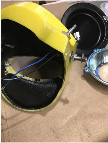
I also decided it would be much easier to install the microswitches before re-installing the pods back on the car. These switches ensure that the lights are not left on when the pods are in the closed position and on the other side they trigger the relay flasher when the pods are raised with the main light switch off.
