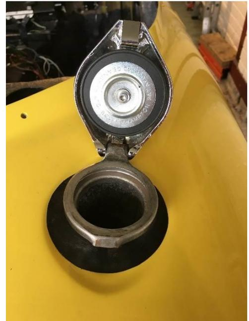
However, most of the problems were overcome by using some extra large washers and a more flexible rubber filler connector than supplied by PM. Fitting the spare wheel in the residual space was always a problem but the combination of brand new tread, 155 vs 145 tyres, and tank position means that I have had to deflate the spare slightly and will have to carry a footpump in future. Again reported by others.
