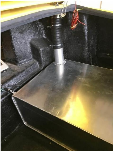
The installation of the fuel tank was delayed as I awaited the return of my re-furbished petrol cap. As I wanted to use my original cap, I managed to drill out the seal rivet, obtain a kit to replace the seal. The cap was then re-chromed and re-assembled.
