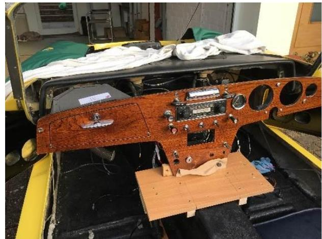
To help hold the dashboard stable whilst attaching the wiring to switches etc., I made a "table" (see photo) for the dashboard to sit on.
