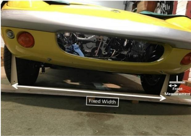
I created a fixed measuring “tool” from a length of wood and two upright shelf brackets with the distance between the uprights at about 10 cms less than the track width. This enabled me to then measure (separately) the width between front of the tyres and between the rear of the front tyres (mid way across the tread and at hub height). I then adjusted the track rod ends to obtain the required “toe-in” of circa 3 mm.
